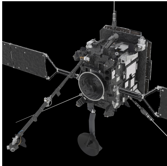
Fig. 15. Rear view of the Solar Orbiter spacecraft. The instrument boom hosts the SWA/EAS sensor at its tip, and the RPW/SCM sensor as well as the two MAG sensors along its length. The high-gain antenna is made out of titanium treated with SolarBlack , and is fully articulated to communicate with ground stations throughout the orbit. The rear-side of the solar arrays has been covered with conductive foil to avoid electrostatic charging.
