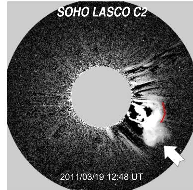
Figure 9. SOHO/LASCO/C2 difference image during event 2 showing a CME with two different structures. The CDAW speed was estimated using the southern structure indicated by the white arrow, whereas the angular width was estimated combining the two well-differentiated structures.
