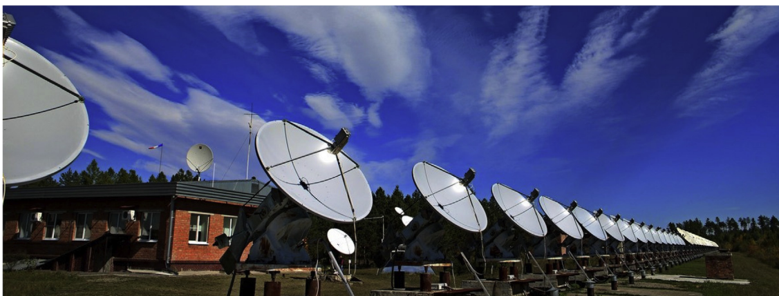
Fig. 2. View of the 48-antenna SRH first stage (the east arm). White remote larger dishes on the right (east) belong to the old SSRT antenna system. Separate dishes on the ground behind the SRH antennas belong to the total-flux spectropolarimeters (Zhdanov and Zandanov, 2015). The receiver and control systems are located in the working building visible behind the SRH antennas on the left.
