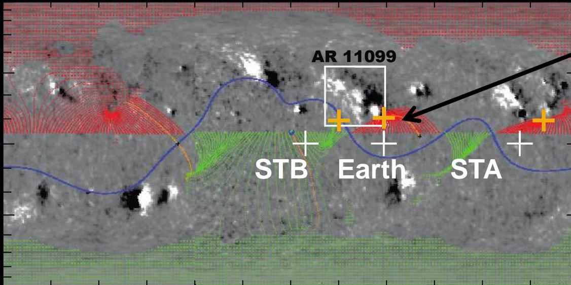
The magnetic footpoints of three spacecraft calculated by Parker spiral field formula considering solar wind speed.
