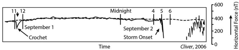
**Figure 1.** Magnetogram (adapted from Cliver [2006]) of the horizontal component of the magnetic field obtained by Stewart [1861] in London in 1859. Dashed line represents the quiet day variation.
