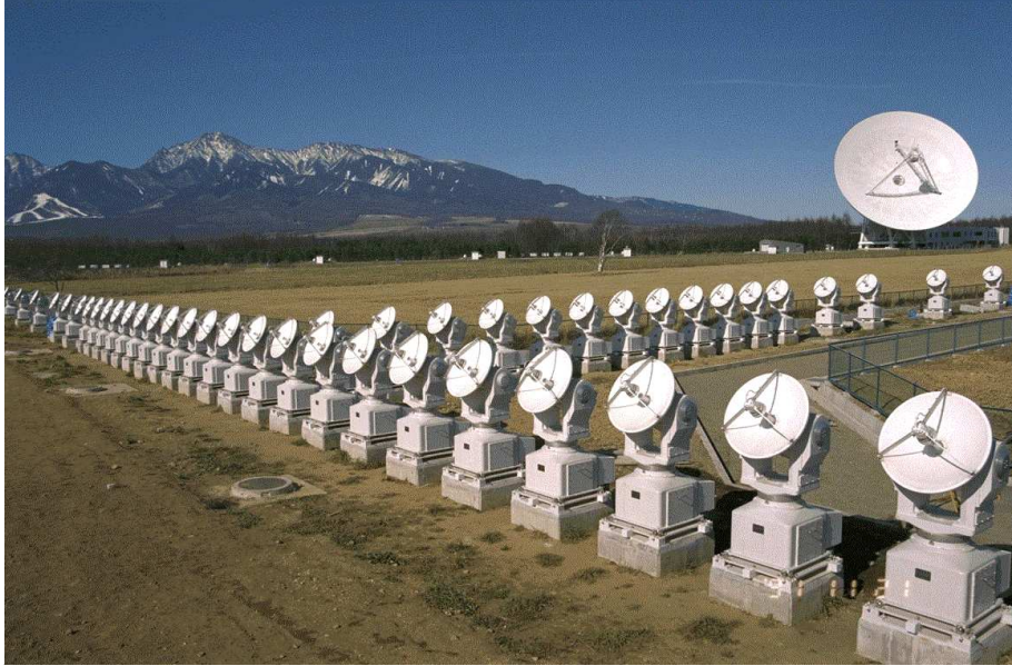
Figure 1.15: The Nobeyama Radioheliograph (NoRH) in Japan, consisting of 84 parabolic antennas with 80 cm diameter, arranged in two arms, one with a length of 490 m in east/west direction, the other with a length of 220 m in north-south direction. First observations were made in April 1992, and are continued already over 20 years (Credit: NRO/NAO).
