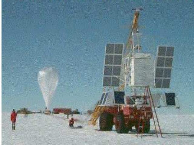
Figure 1.14: HIREGS large balloon-borne X-ray and gamma-ray detectors to observe solar flares and astrophysical high-energy sources, launched by the Univ. Berkeley Space Physics Research Group (principal investigator Bob Lin), circum-navigating Antarctica from November 1994 to January 1995 (Credit: Univ. Berkeley SPR).
