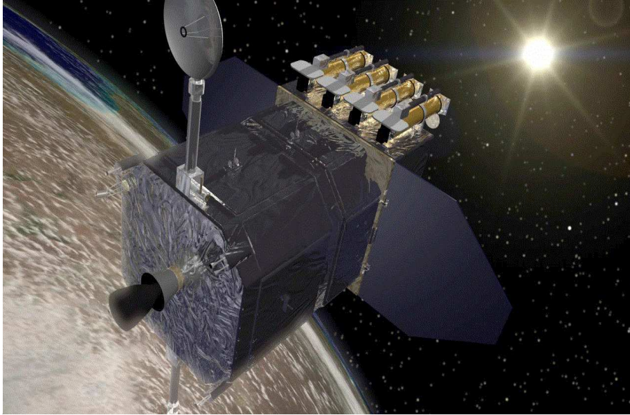
Figure 1.10: The Solar Dynamics Observatory (SDO) spacecraft is shown in an artist's impression. The four golden tubes represent the four Atmospheric Imaging Assembly (AIA) telescopes (Courtesy NASA and SDO Team).
