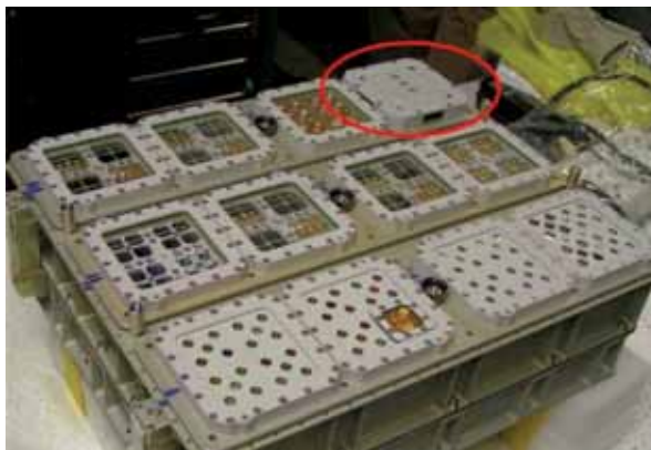
Figure 2. External view of the EXPOSE-R facility. The R3DR instrument was situated inside of the red oval. EXPOSE-E facility was with very similar external view
