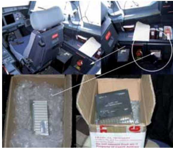
Figure 1. Position of the Liulin detector inside the Airbus' cockpit
