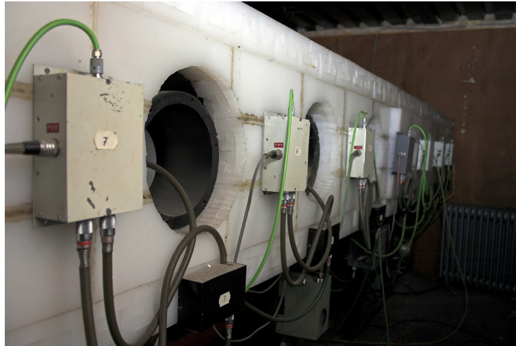
Fig. 3.7. Lomnický štít neutron monitor since 1981 measures with 8 proportional counters of the type SNM 15. The statistics is \sim 1.6 \times 10^6 counts/hour. The detail shows a reflector, moderator and partially one counter. More informations about the measurements of CR in High Tatra mountains can be found e.g in paper [Kudela & Langer, 2009].
