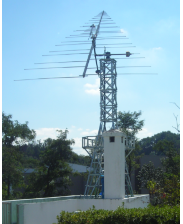
Fig. 2. — The log periodic dipole antenna of the station. It is mounted horizontally on an azimuth/elevation mount on top of a 6 m high tower. CALLISTO receiver is located in a steel case underneath the tower and remotely controlled from the nearby observatory using RS-422 link.
