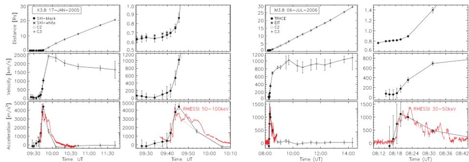
**Figure 1b:** Left: CME dynamics for the 2005 January 17 X3.8 flare/CME event. Right: CME dynamics for the 2006 July 6 M3.8 flare/CME event. The acceleration of the CMEs and the RHESSI HXR flux are closely synchronized within about 5 min. The peak acceleration of about 5 km/s<sup>2</sup> and 1.3 km/s<sup>2</sup> occurs at a plane-of-sky distance from the Sun center <1 Rs.
