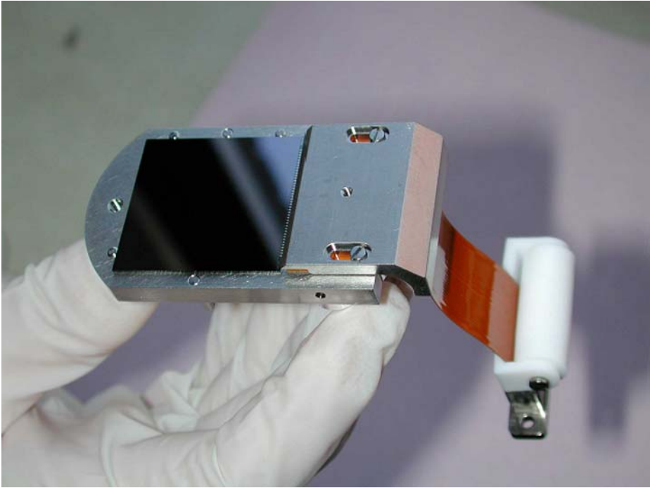
Fig. 24 SECCHI CCD in its package with flexprint harness attached. The CCD size is 28.1 mm \times 30.3 mm
