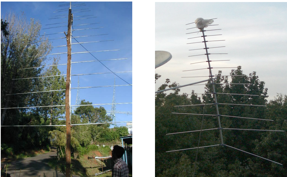
Fig. 3: Logarithmic periodic antennas of e-CALLISTO. Left: at Ootacamund (Ooty) in Tamil Nadu, India; Right: at UNAM, Mexico D. F.
