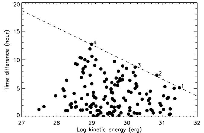
FIG. 5.—Variation of the CME-noise storm onset time difference with kinetic energy of the CME. The straight line (obtained using points numbered 1, 2, 3, and 4) indicates the cutoff in the above time interval for different values of CME kinetic energy.
