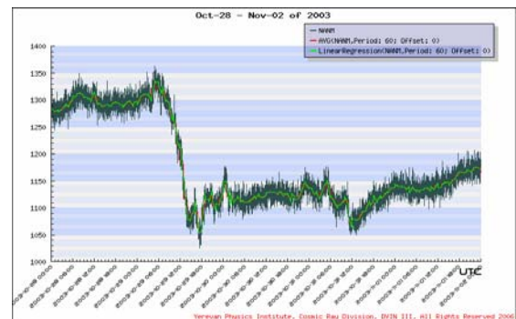
Figure 8 Average (red) and Linear Regression (green) interpolation of the Nor Amberd neutron monitor time series.
