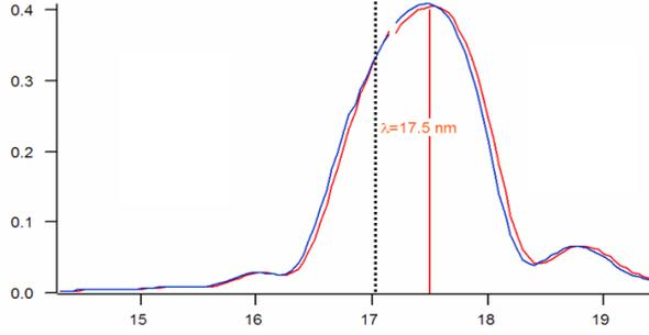
Fig. 2. Reflectivity (1 bounce) provided by the multilayer coating on a test sample. The bandpass is  $\tilde{1}.3$  nm, with peak reflectivity of 40.5 % (source: IOTA). The separation between the two lines correspond to the range of incidence angles on the mirror (1 and 4 degrees). The dashed line outlines the aluminum cut-off of the front filter below which no photons enter the telescope.
