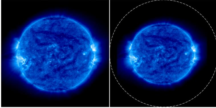
Fig. 4. The 20 % larger field of view of SWAP is shown on the right. The circle corresponds to 1.67 solar radii. The corners of the SWAP field of view correspond to 2.36 solar radii. On the left we show for comparison the original EIT image that was used as input.
