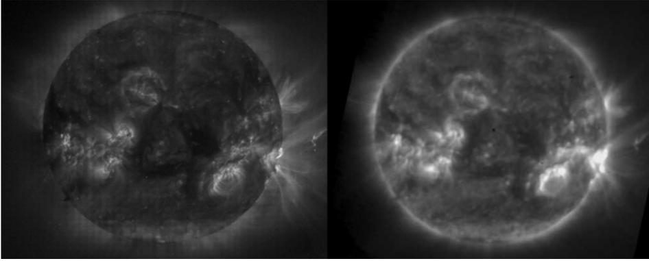
Fig. 3. EIT 19.5 nm bandpass (left) compared with SPIRIT 17.5 nm bandpass (right) with only 25 sec difference in observation time. The dynamic range in the EIT 19.5 nm bandpass is slightly larger than in the SPIRIT 17.5 nm bandpass (e.g. the contrast between active regions and coronal holes). Both images show an ejection at the right hand side of the image.
